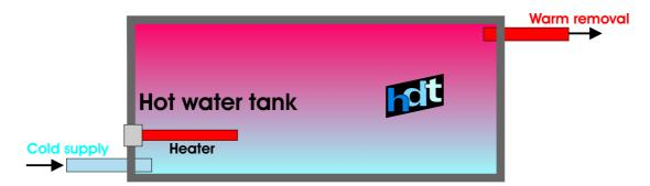
A significant amount of hot water can be taken from a tank before it gets cold (depending on the volume of the tank). Although the inflow of cold water is  $10\,^\circ$  C, hot water still comes out at the top. In this case we want to remove the heat with the water. Imagine you had to stand under a shower where the tank functioned the other way around.
